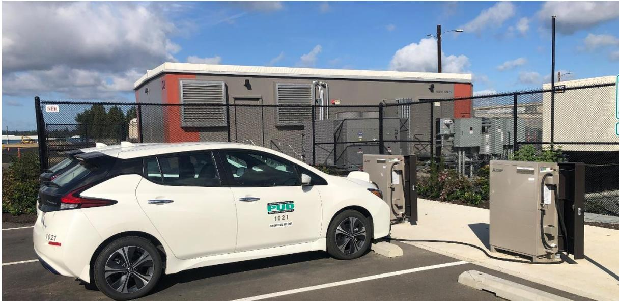
Figure 3 : These light-duty electric vehicles charge and discharge power into the Arlington microgrid and PUD grid
