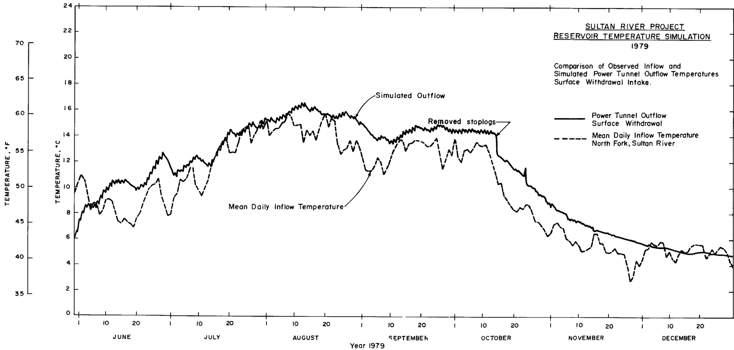
Figure 4-10 Comparison of the Observed Spada Lake Inflow Temperatures with the Simulated Power Tunnel Outflow Temperatures, Surface Withdrawal Intake, 1979
