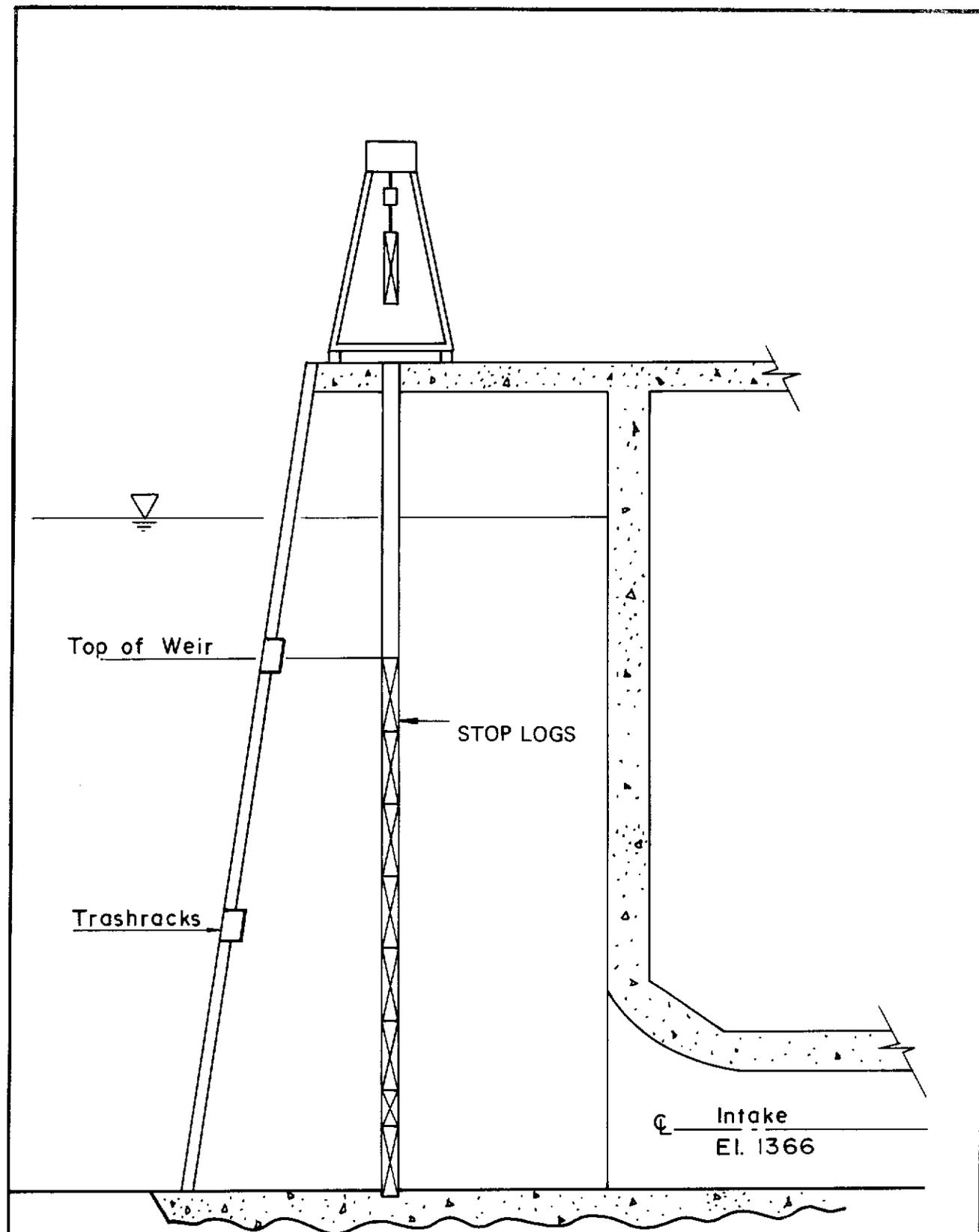
Figure 4-5 Conceptual Layout of a Surface Withdrawal Intake
