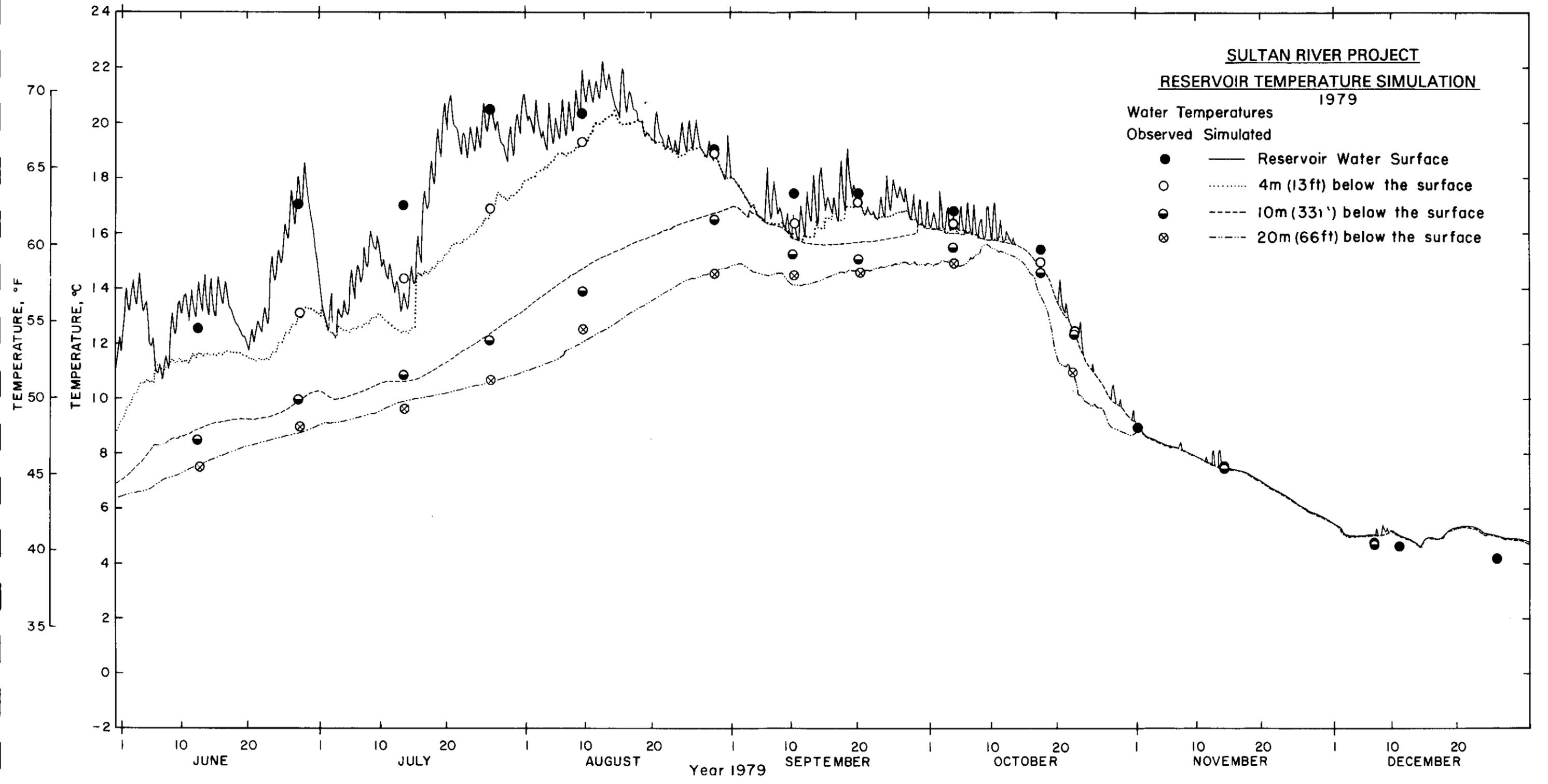
Figure 3-5 Comparison of Observed and Simulated Temperatures in Spada Lake, June-December 1979
