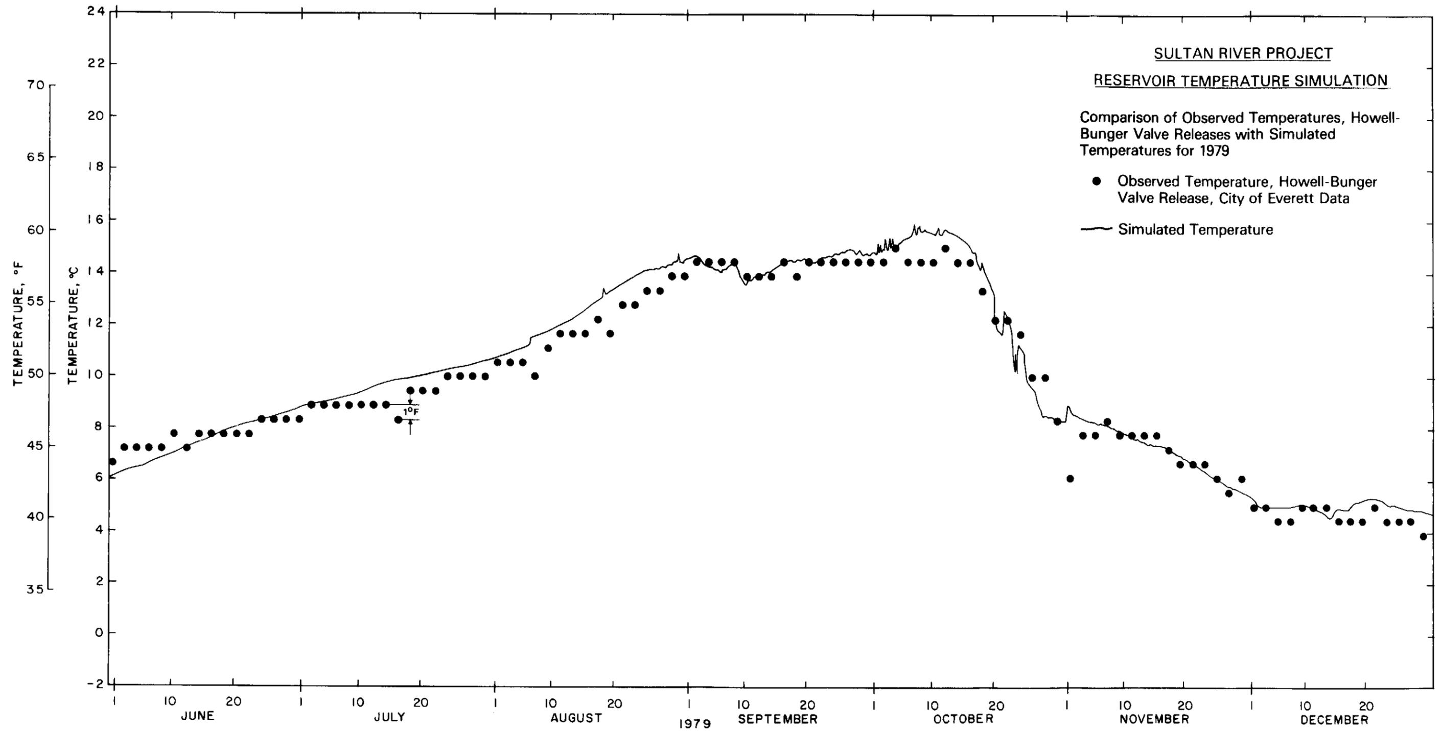
Figure 3-9 Existing Reservoir Outlet Temperatures: Simulated Temperature of Howell-Bunger Valve Releases and City of Everett Observed Temperatures, 1979
