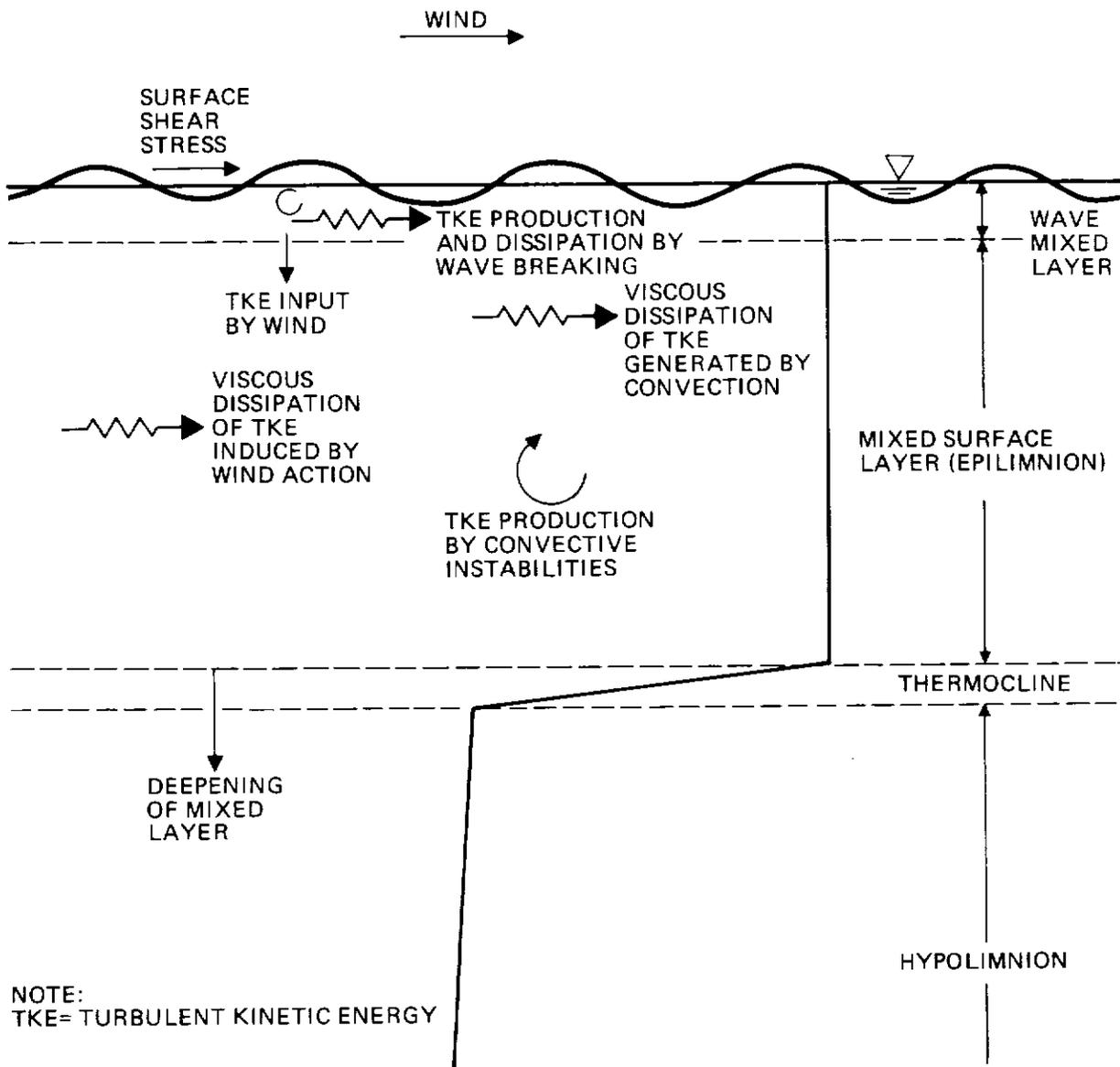
**Figure 3-2 Definition Sketch: Physical Processes Affecting the Growth of the Wind-Mixed Surface Layer**
