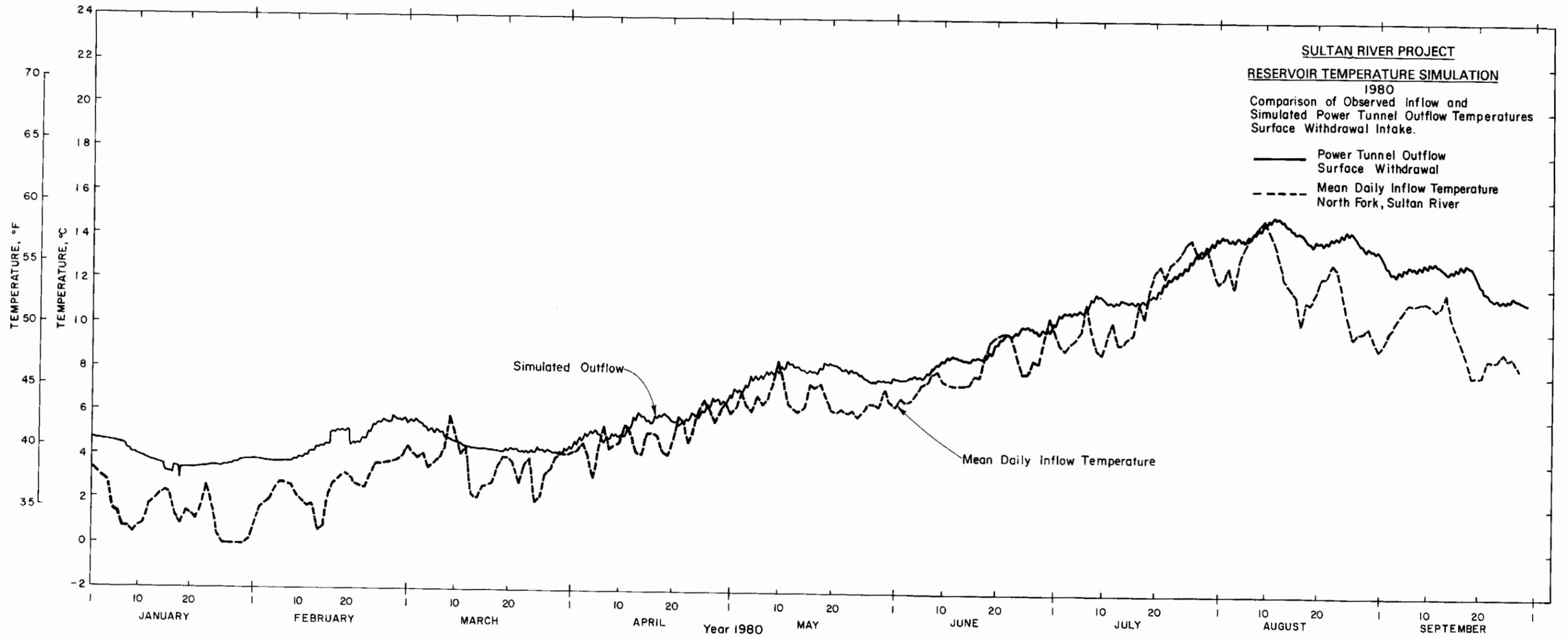
Figure 4-11 Comparison of the Observed Spada Lake Inflow Temperatures with the Simulated Power Tunnel Outflow Temperatures, Surface Withdrawal Intake, 1980
