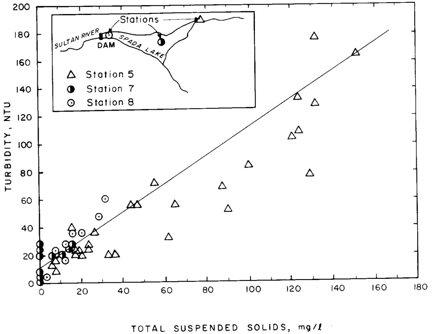
Figure 3-4 Relationship Between Turbidity and Suspended Solids Concentration
