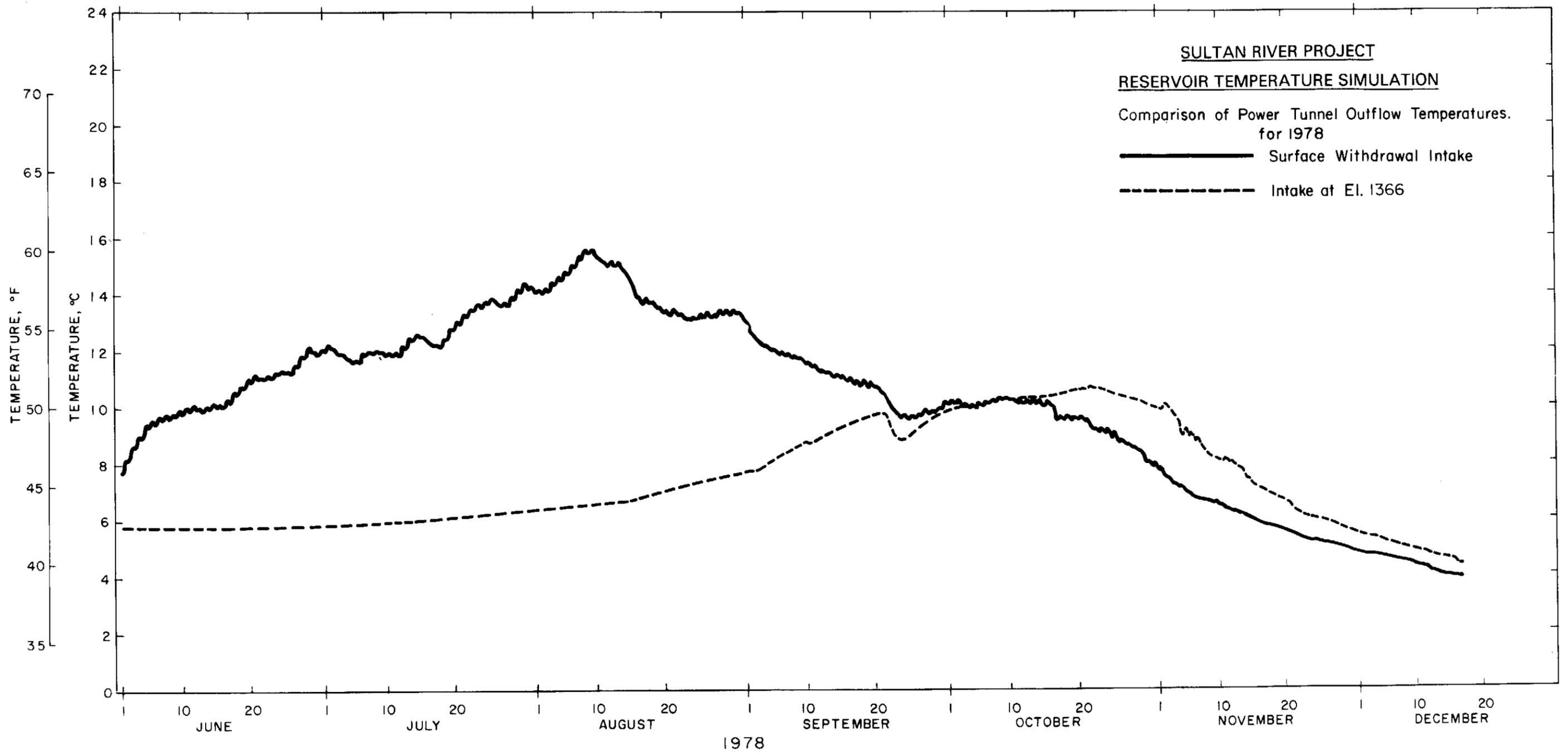
Figure 4-7 Comparison of Power Tunnel Outflow Temperatures, Surface Withdrawal Intake and Intake at Elevation 1,366, 1979
