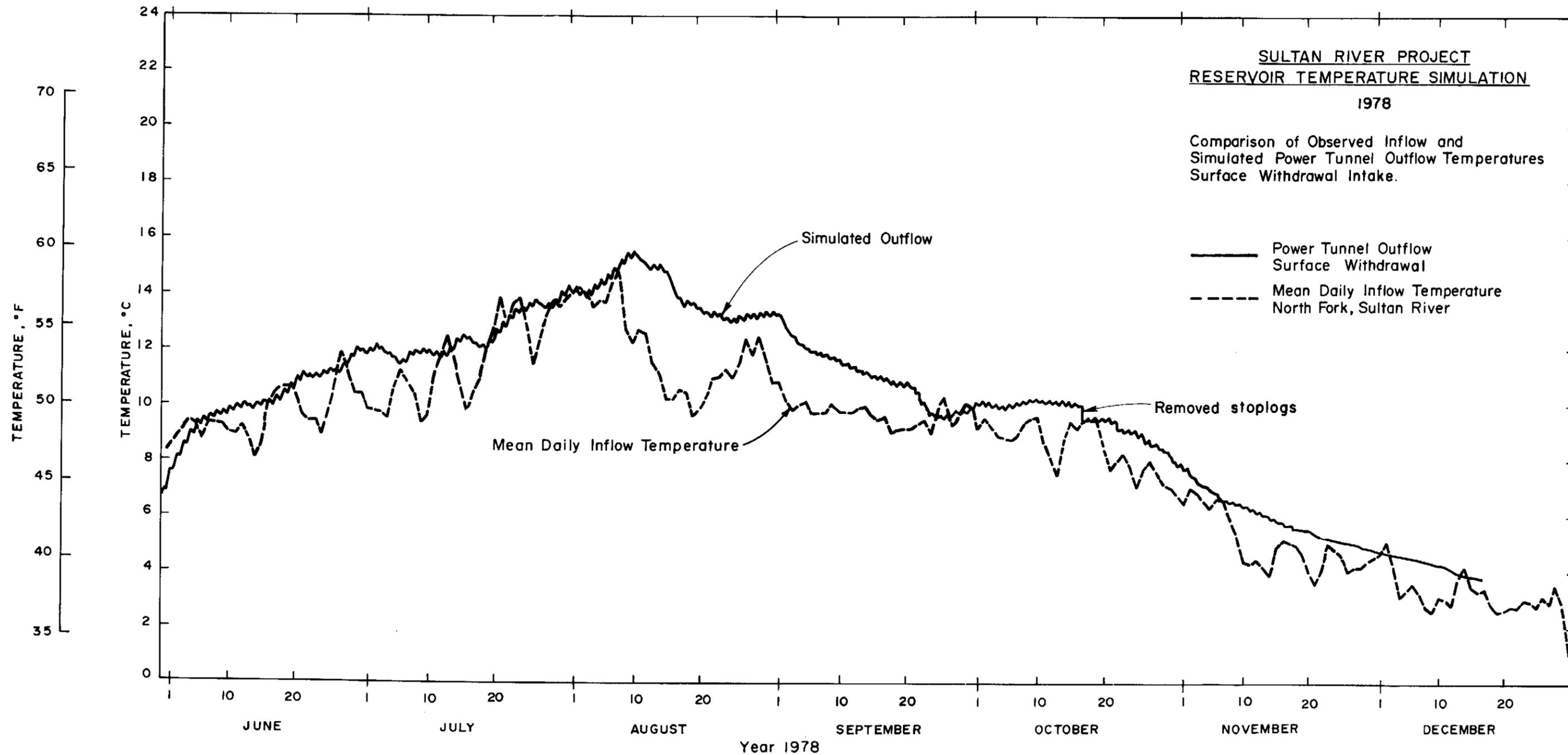
**Figure 4-9** Comparison of the Observed Spada Lake Inflow Temperatures with the Simulated Power Tunnel Outflow Temperatures, Surface Withdrawal Intake, 1978
