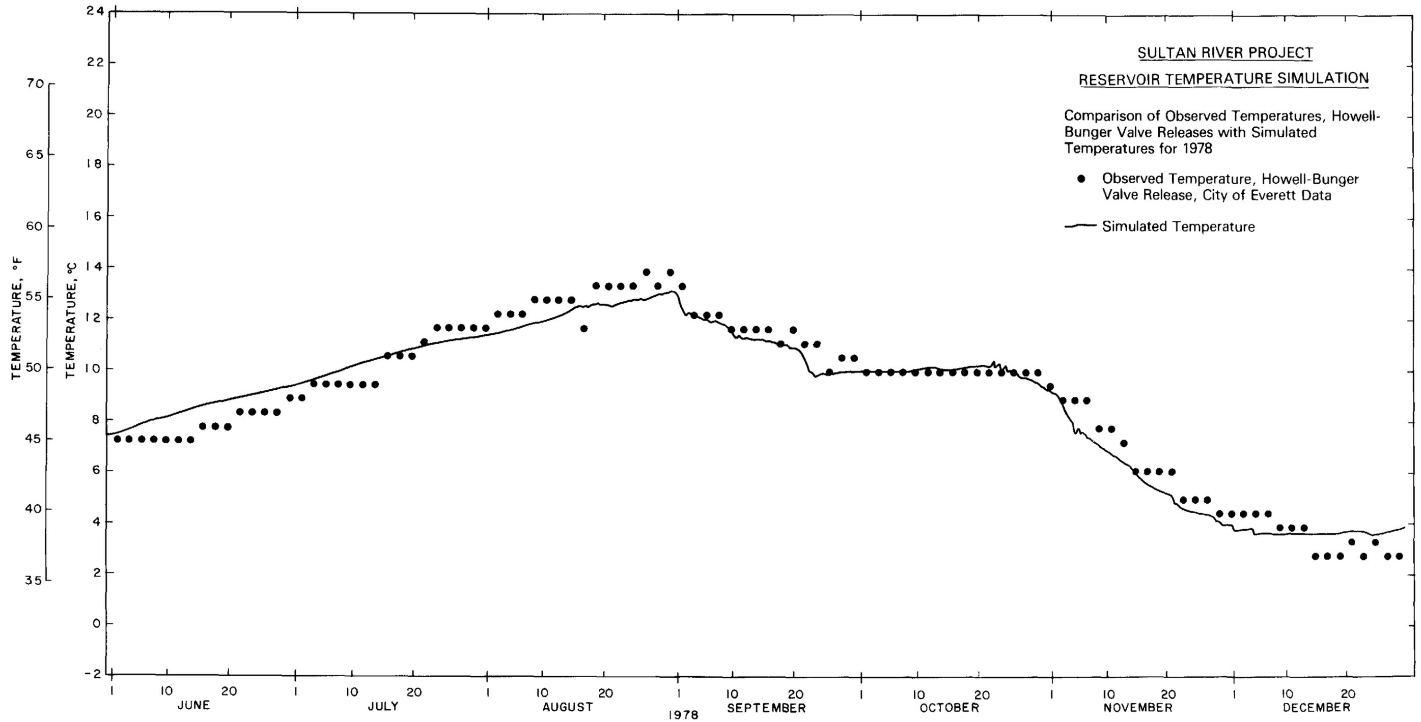
**Figure 3-14 Existing Reservoir Outlet Temperatures: Simulated Temperature of Howell-Bunger Valve Releases and City of Everett Observed Temperatures, 1978**
