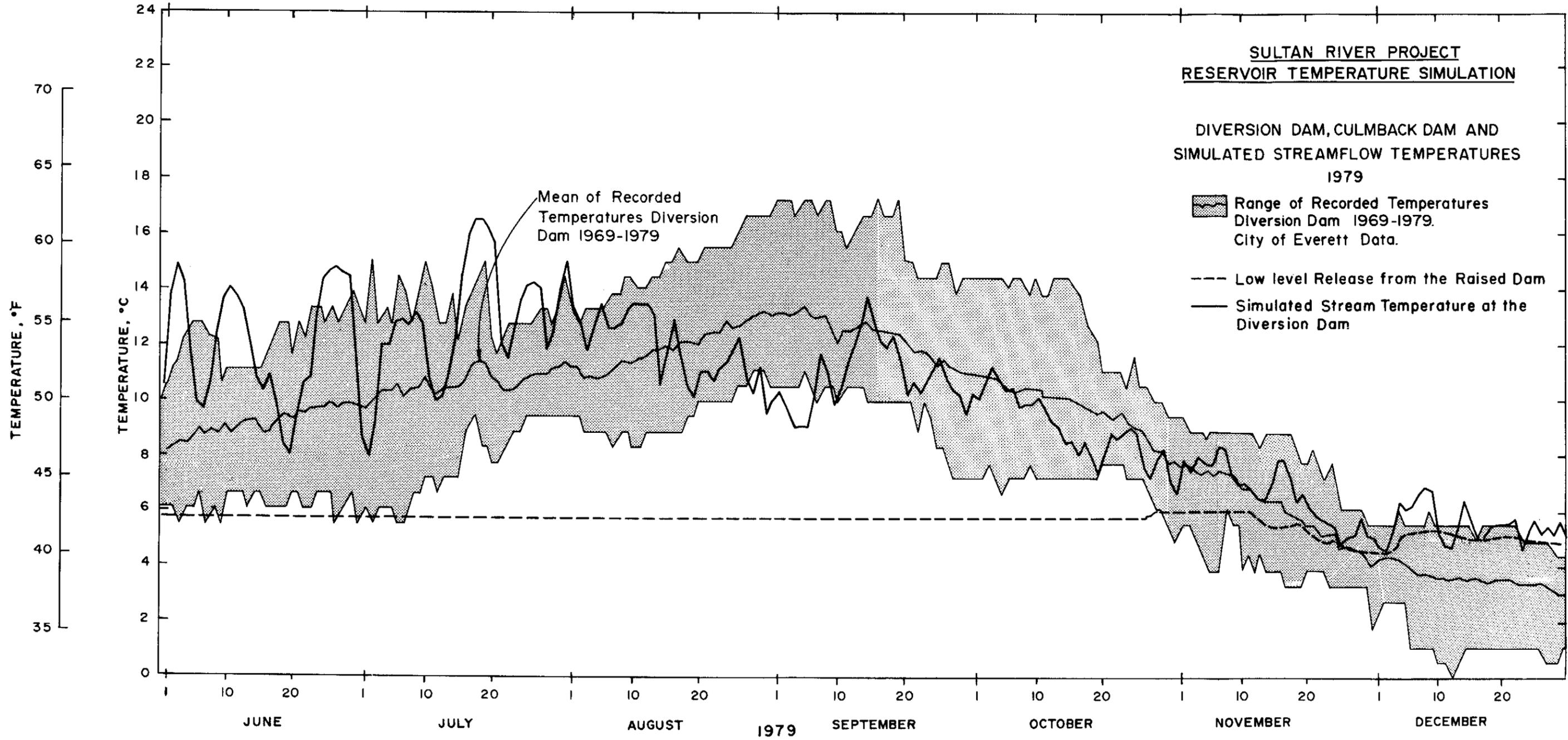
**Figure 4-13 Streamflow Temperature Model.**
