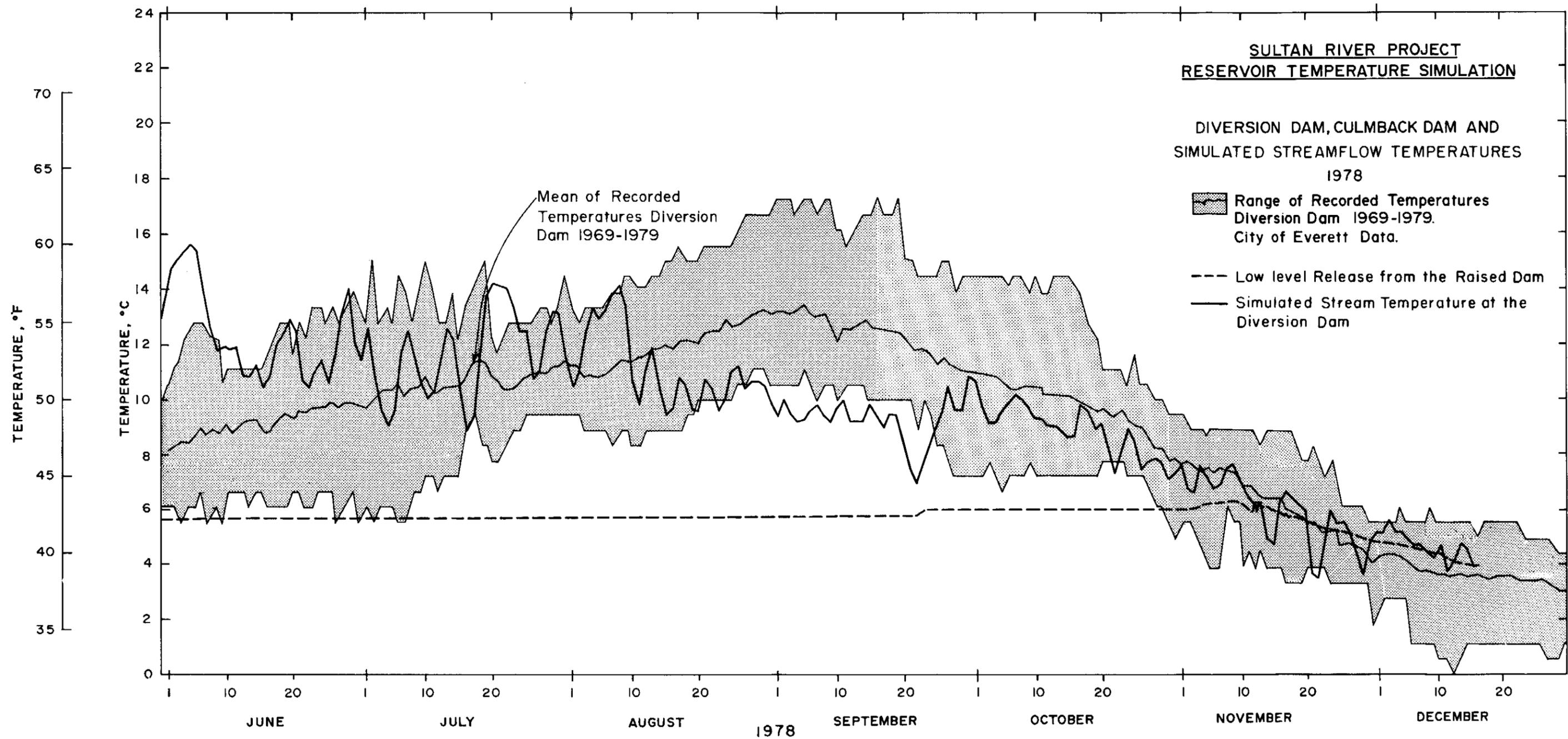
**Figure 4-12 Streamflow Temperature Model.
