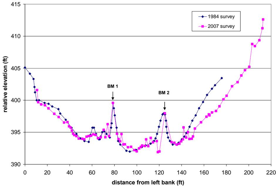
**Figure 2-6** Cross-section comparison at the Upper Site. Elevation is relative to the BM 1 and BM 2 elevations derived from the 1984 GeoEngineers survey plot.
