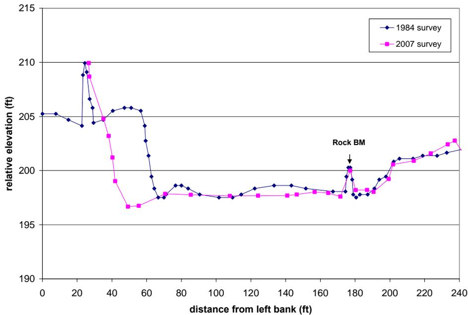
**Figure 2-2 Cross-section comparison at the Kien's Bar Site, XS 1.** Elevation is relative to the Rock BM elevation (200 ft) given in the 1984 GeoEngineers survey.
