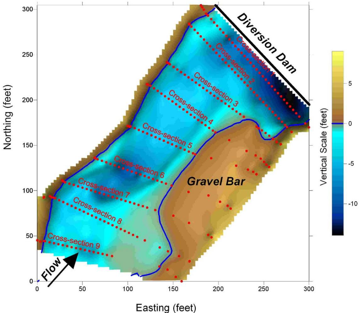
**Figure 2-7 Reservoir bathymetry for the sediment deposit behind the Diversion Dam (July 2007). The solid blue lines indicate the water surface elevation at the time of measurement.**
