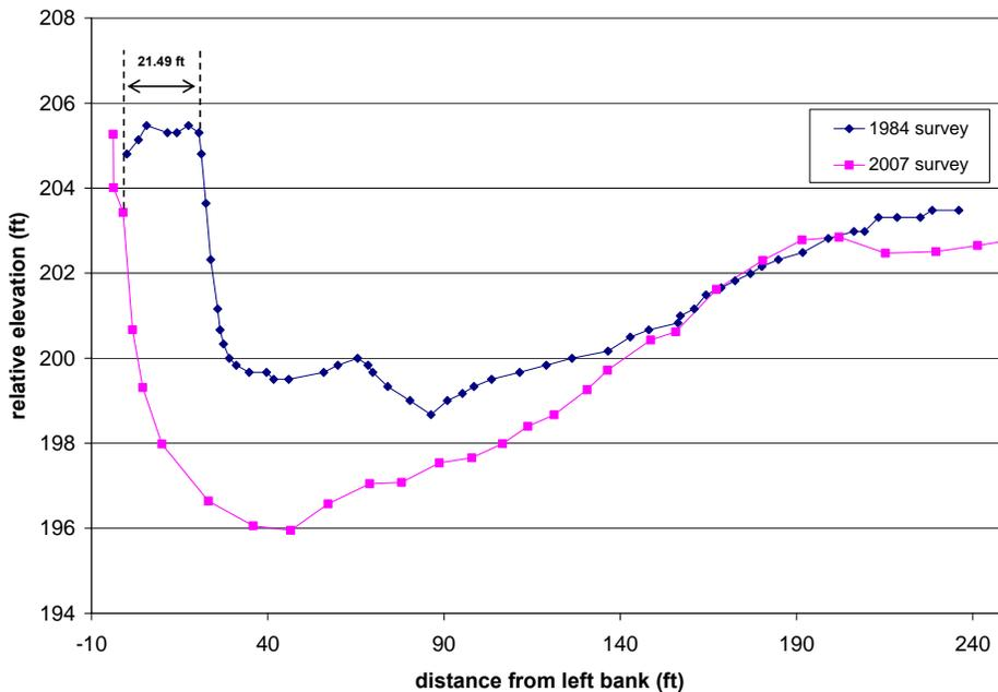
**Figure 2-4 Cross-section comparison at the Kien's Bar Site, XS 3.** Elevation is relative to the Rock BM elevation (200 ft) in XS 1. Due to the lack of surveying benchmarks at this location from the 1984 GeoEngineers survey, the two cross-sections were aligned in the horizontal based on the measured bank retreat of 21.49 ft at XS 1.
