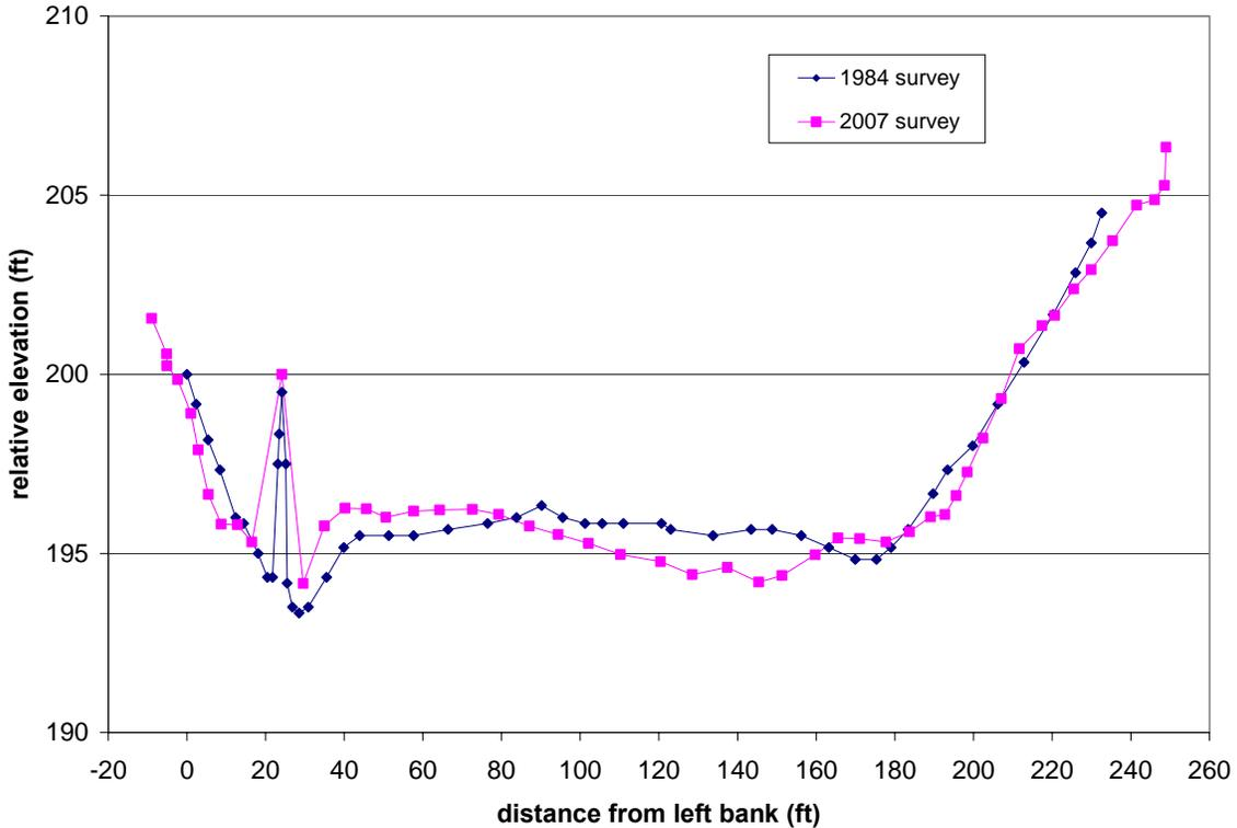
**Figure 2-5 Cross-section comparison at the Chaplain Site.** Elevation is relative to the Rock BM elevation (200 ft) given in the 1984 GeoEngineers survey.
