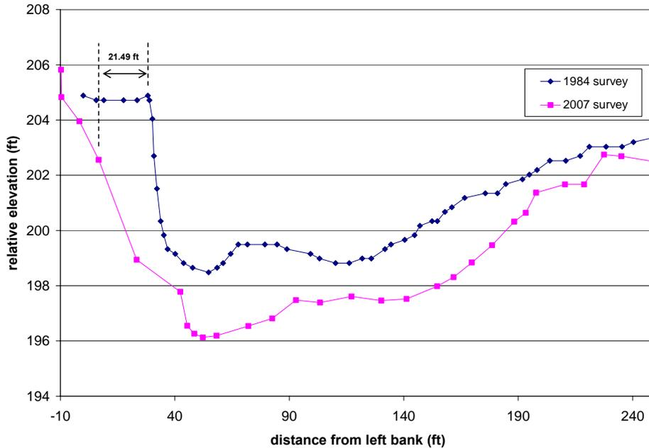
**Figure 2-3 Cross-section comparison at the Kien's Bar Site, XS 2.** Elevation is relative to the Rock BM elevation (200 ft) in XS 1. Due to the lack of surveying benchmarks at this location from the 1984 GeoEngineers survey, the two cross-sections were aligned in the horizontal based on the measured bank retreat of 21.49 ft at XS 1. Note change in Y-axis scale relative to Figure 2-2.
