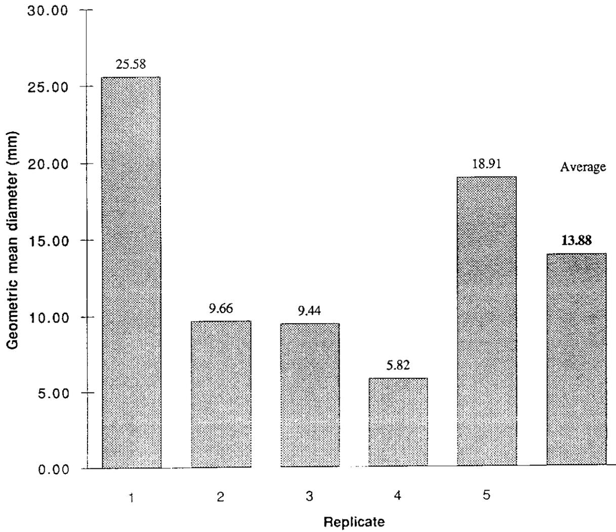
**Geometric mean diameter - volumetric (DGW) using all four strata for each replicate at Station 5B on the Sultan River for 1994**
