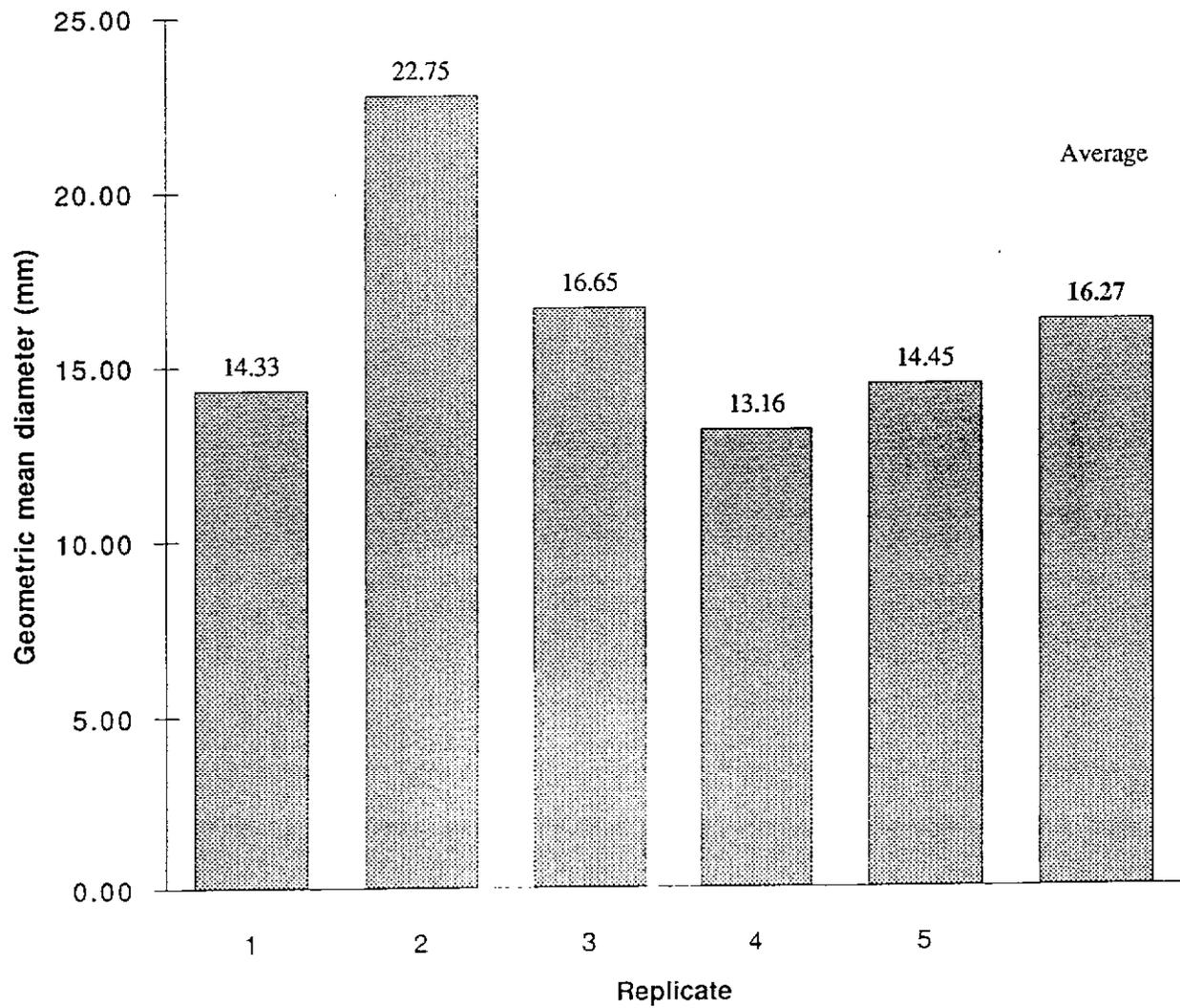
**Geometric mean diameter - volumetric (DGW) using all four strata for each replicate at Station 2 on the Sultan River for 1994**
