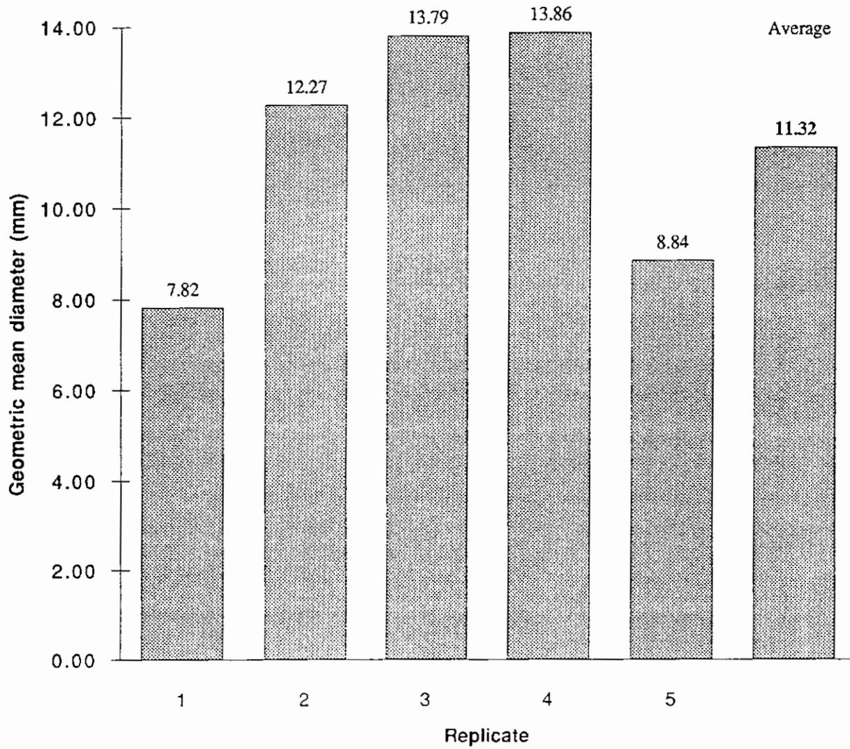
**Geometric mean diameter - volumetric (DGW) using all four strata for each replicate at Station 3 on the Sultan River for 1994**
