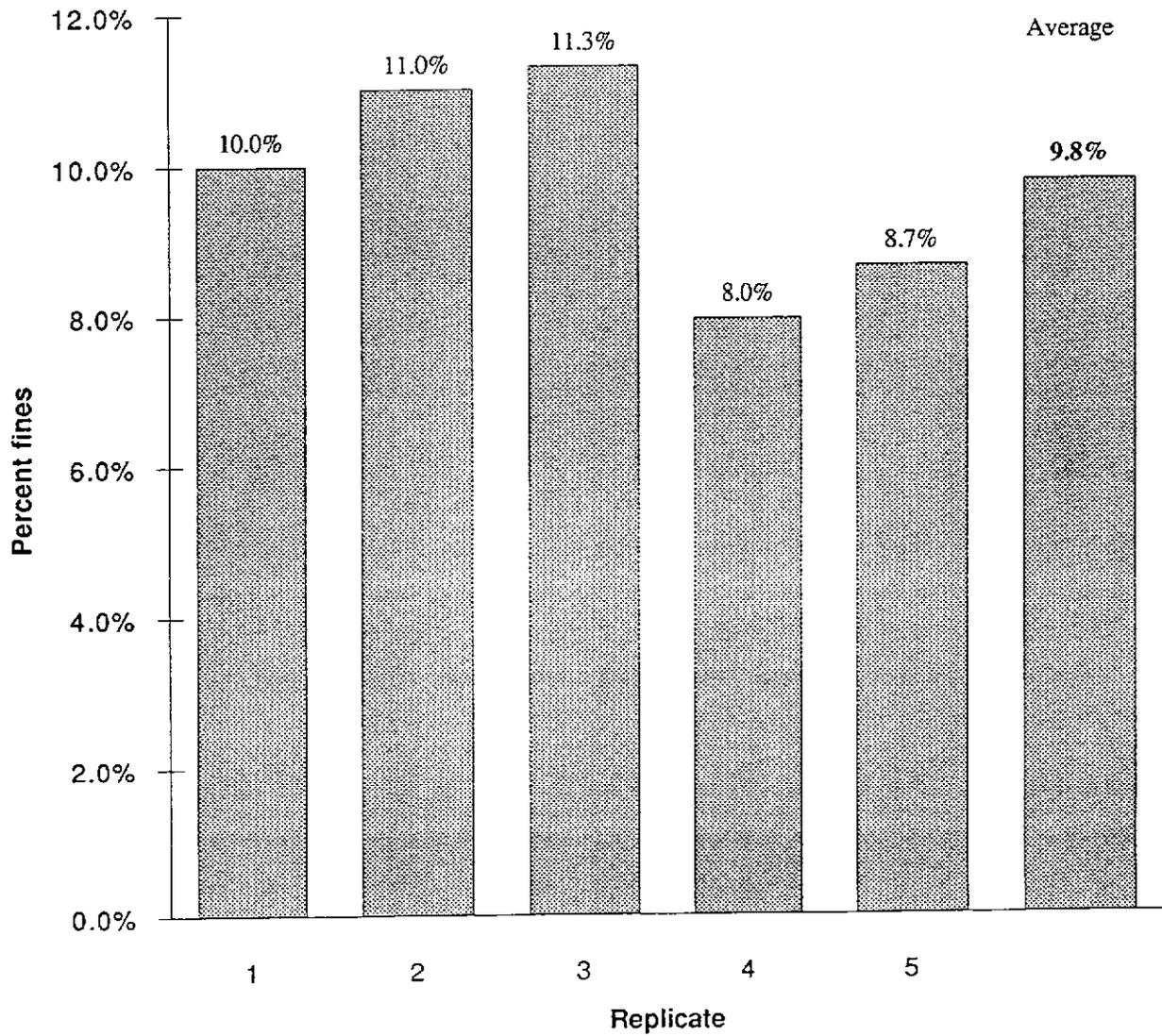
**Percent fines - volumetric (PFW) using all four strata for each replicate at Station 3 on the Sultan River for 1994**
