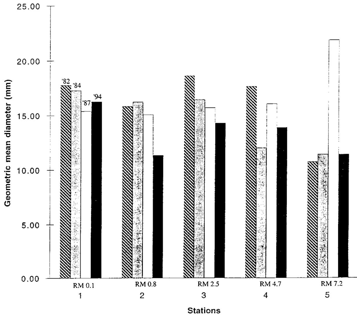
**Average geometric mean diameter (DGW - volumetric) for all four strata at each station (S1-S5) on the Sultan River for each year of the study**
