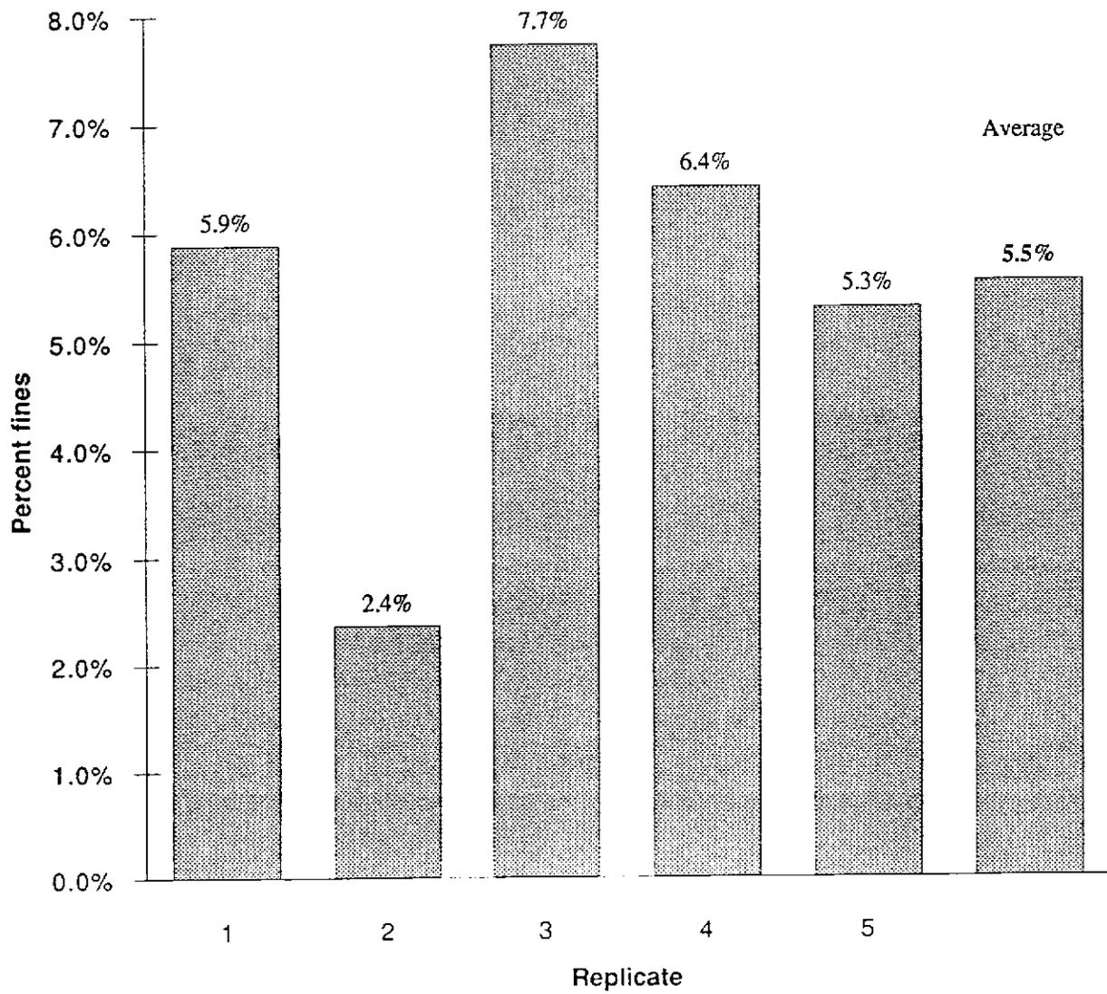
**Percent fines - volumetric (PFW) using all four strata for each replicate at Station 2 on the Sultan River for 1994**
