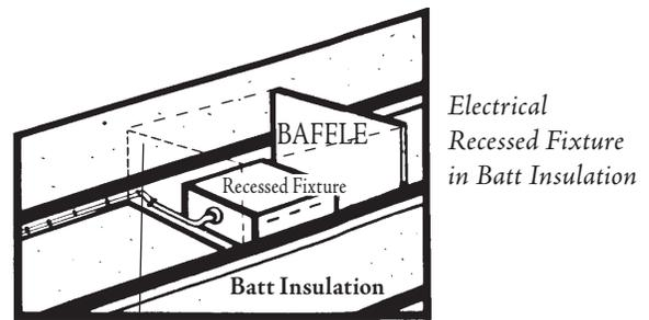
NOTE: Tops of baffle need to be above the final level of insulation.
