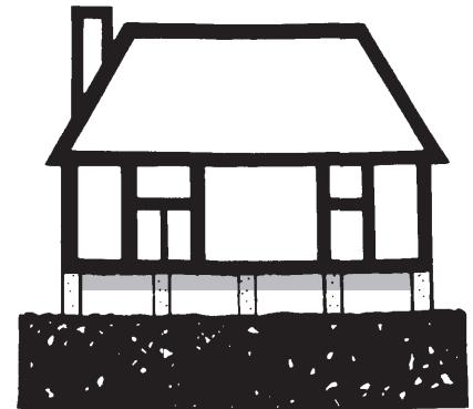
Floor over crawl space
